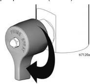
If you suspect that the spray tip or hose is completely clogged, or that pressure has not been fully relieved after following the steps above, VERY SLOWLY, loosen tip guard retaining nut or hose end coupling to relieve pressure gradually, then loosen completely. Then clean tip and hose.
